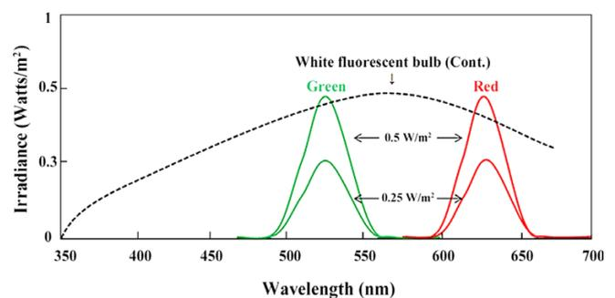
**Fig. 1.** Spectral profiles of light emitting diodes (LEDs; green, 520 nm; red, 630 nm) and white fluorescent bulb (Cont.) used in this study. Each LED light source was set at two intensities (low, 0.25 and high, 0.5 W/m<sup>2</sup>). Reprinted from Shin et al. (2011), with permission from Comparative Biochemistry and Physiology, Part-A
